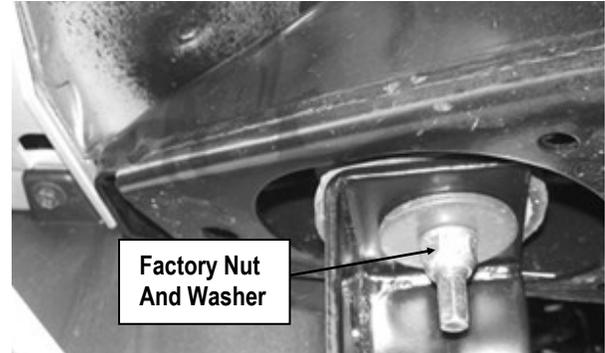
(Fig 2) Driver Rear Mounting Bracket Installation
