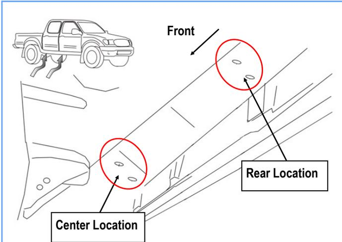
(Fig 3) Passenger Center And Rear Mounting Location
