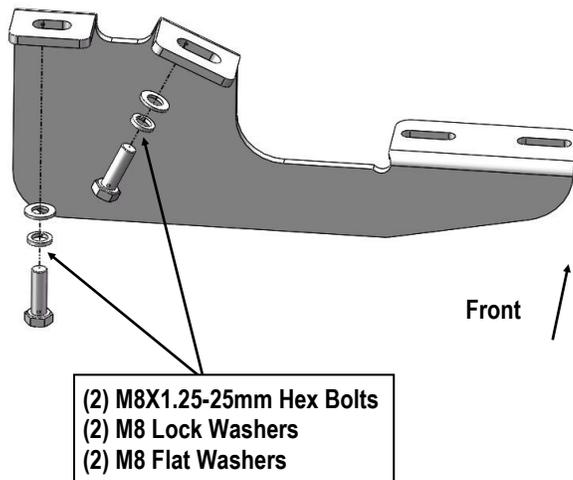
**(Fig 2) Passenger Front Mounting Bracket Installation**
