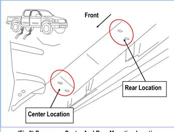
(Fig 3) Passenger Center And Rear Mounting Location
