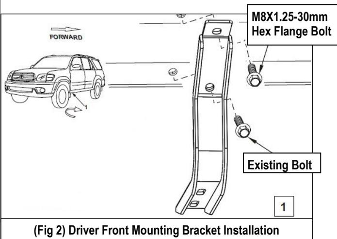
(Fig 2) Driver Front Mounting Bracket Installation
