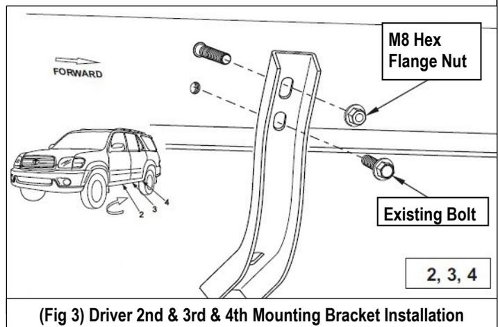
(Fig 3) Driver 2nd & 3rd & 4th Mounting Bracket Installation
