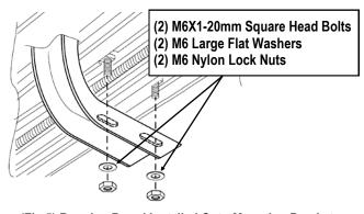
(Fig 5) Running Board Installed Onto Mounting Bracket
