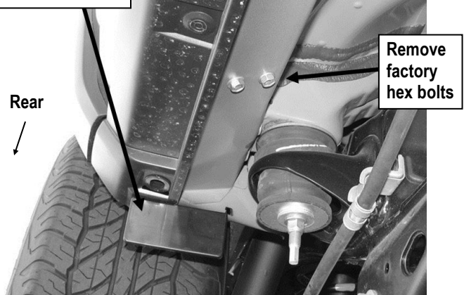
(Fig 3) Passenger Side Rear Mounting Location
