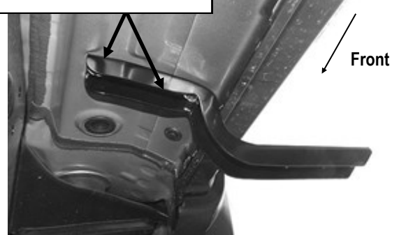
(Fig 2) Passenger Front Mounting Bracket Installed
