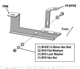
(Fig 5) Passenger Side Rear Mounting Bracket Assembly
