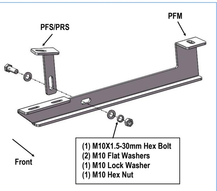
(Fig 2) Passenger Side Front Mounting Bracket Assembly
