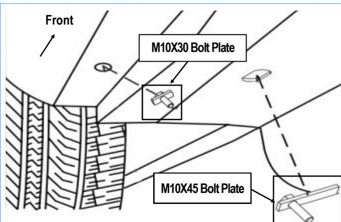
(Fig 4) Passenger Side Rear Mounting Location
