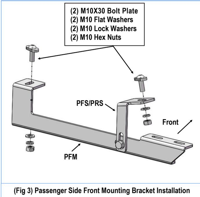
(Fig 3) Passenger Side Front Mounting Bracket Installation
