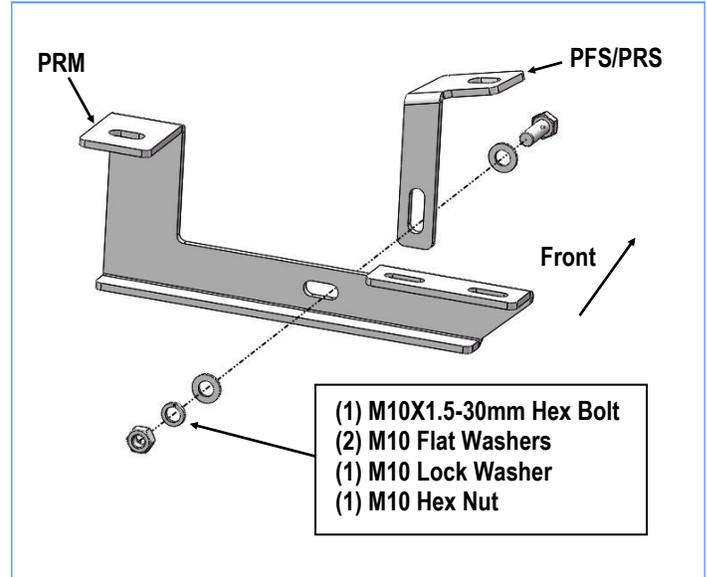
(Fig 5) Passenger Side Rear Mounting Bracket Assembly
