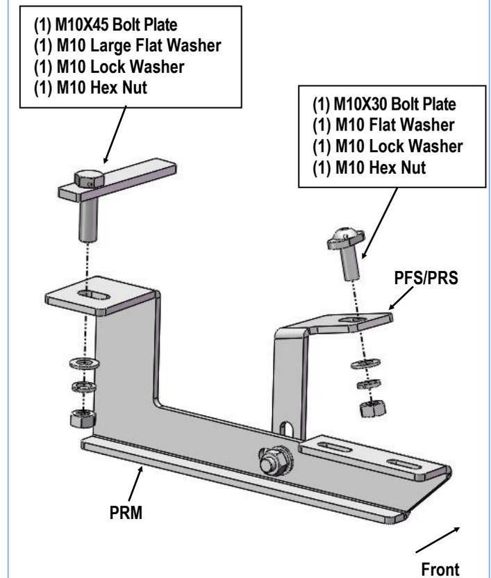
(Fig 6) Passenger Side Rear Mounting Bracket Installation
