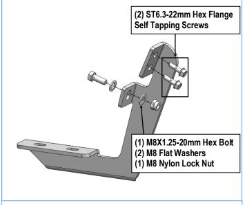
(Fig 2) Driver Front Mounting Bracket Installation
