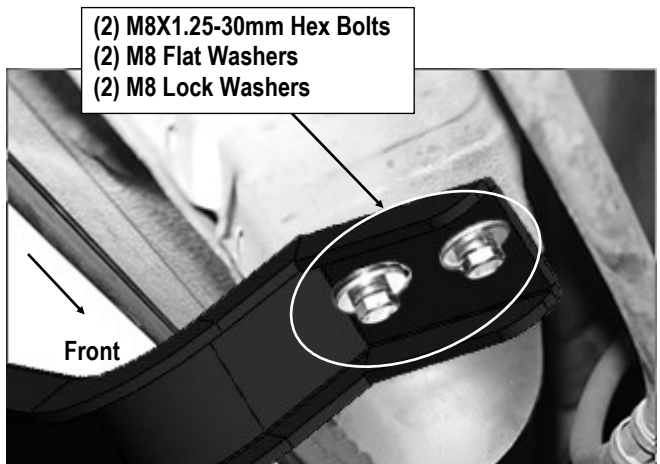
(Fig 4) Driver Rear Mounting Bracket Installation
