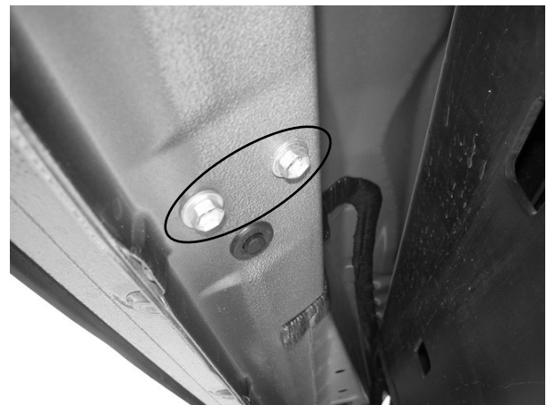
(Fig 3) Driver Center Mounting Location Pictured
