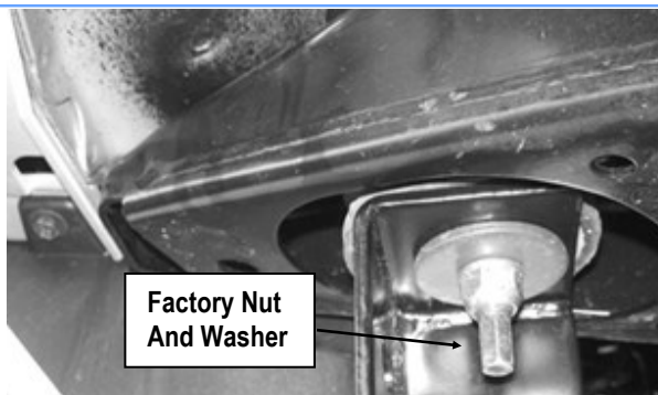
(Fig 2) Driver Rear Mounting Bracket Installation
