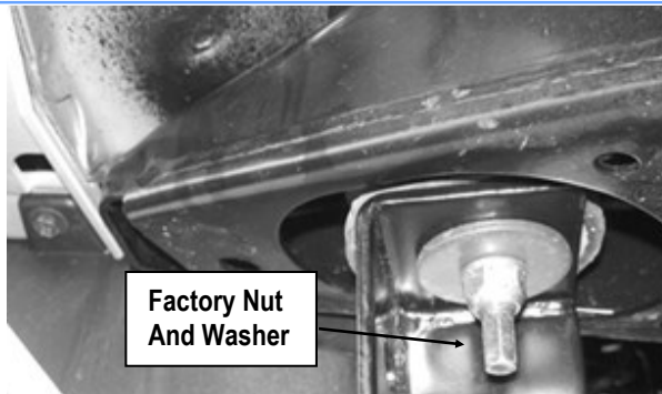
(Fig 2) Driver Rear Mounting Bracket Installation
