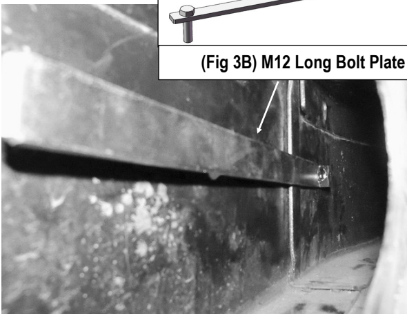
(Fig 3A) Inside View Of M10 Long Bolt Plate Installed (In Driver Side Frame Channel)
