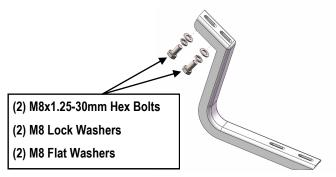
(Fig 4) Driver Center & Rear Mounting Bracket Installed
