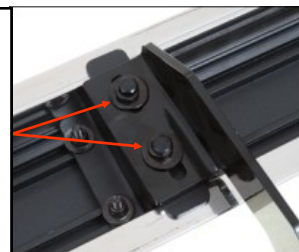
(Fig 11) Step Bar Installed On Bracket Installed
