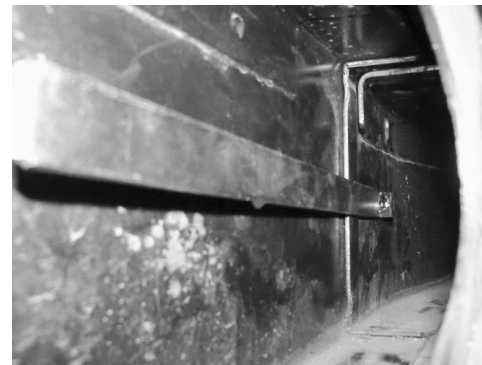
(Fig 3) M12 Long Bolt Plate Installed Inside View (In Frame Channel on Driver Side Front Mounting Location )
