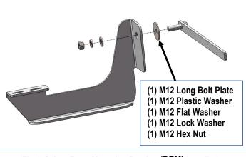
(Fig 4) Driver Front Mounting Bracket (DFM) Installation
