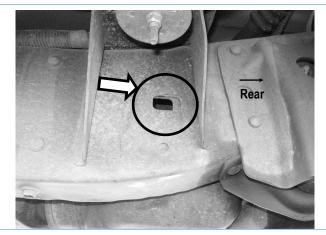
(Fig 5) Driver Side Rear Mounting Location
