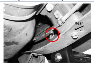
(Fig 6) Driver Rear Mounting Bracket Installed (Back View Of Driver Side-Rear Frame Channel, Reference Only)
