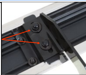
(Fig 19) Step Bar Installed on Bracket Installed (Example)
