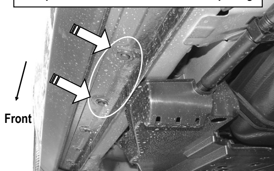
(Fig 7) Driver Side Center Mounting Location
