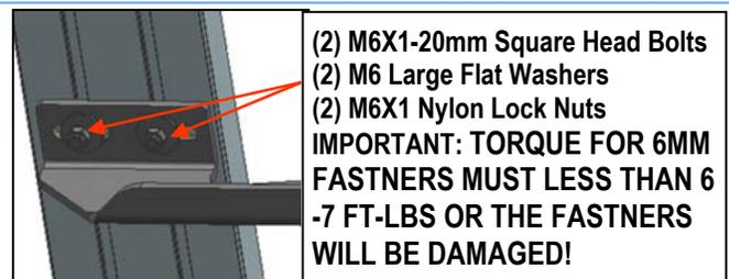
(Fig 7) Running Board Installed Onto Mounting Bracket
