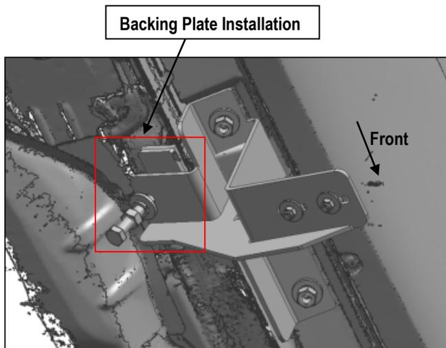
(Fig 5) Passenger Rear Mounting Bracket Installed (Example)
