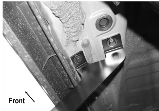
(Fig 3) Passenger Front Mounting Bracket Installed
