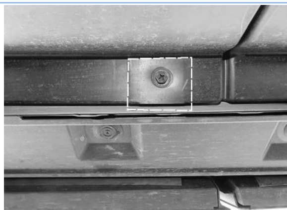
(Fig 5) Passenger Center mounting location, cut along dotted lines
