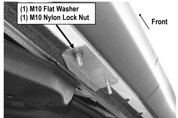
(Fig 10) Locking Plate (DFS1) Installation (Driver Center Side )
