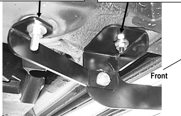
(Fig 6) Driver Side Front Mounting Bracket Installation
