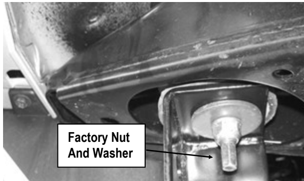
(Fig 2) Driver Rear Mounting Bracket Installation
