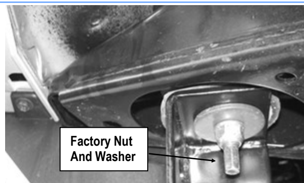
(Fig 2) Driver Rear Mounting Bracket Installation
