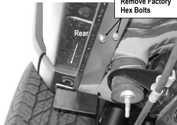
(Fig 3) Passenger Side Rear Mounting Installation
