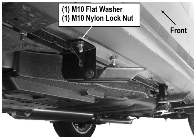
(Fig 7B) Driver Side Front Support Bracket Installation
