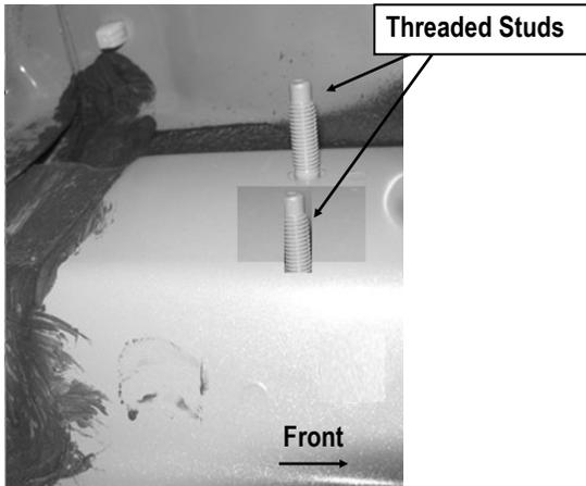
(Fig 1) Driver Side Front Mounting Location Pictured
