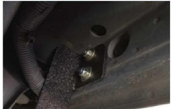
(Fig 3) Driver Side Front Mounting Bracket Installed
