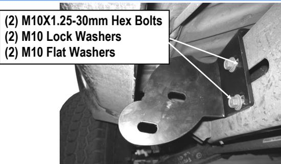
(Fig 2) Driver Front Mounting Bracket (DFM) Installed
