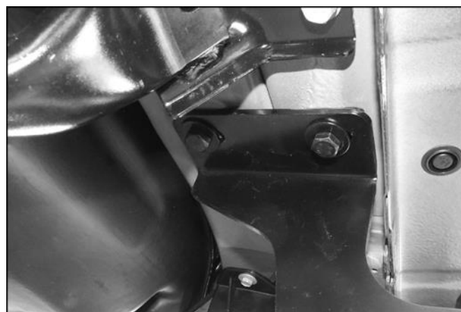
(Fig 8) Driver Rear Mounting Bracket Installed
