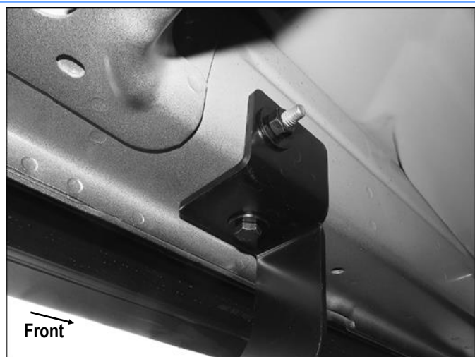
(Fig 5) Driver Center Mounting Bracket Installed
