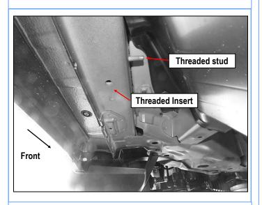
(Fig 1) Driver Side Front Mounting Location
