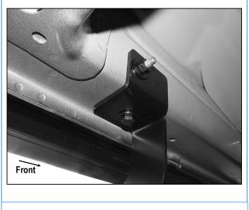
(Fig 5) Driver Center Mounting Bracket Installed
