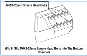
Level and adjust the Running Board and fully tighten all hardware.
