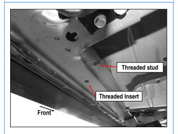
(Fig 4) Driver Side Center Mounting Location
