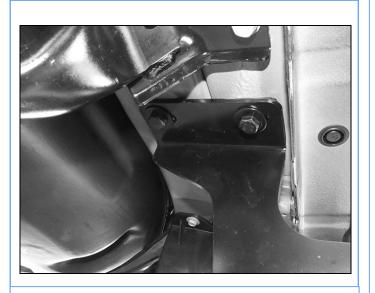
(Fig 8) Driver Rear Mounting Bracket Installed
