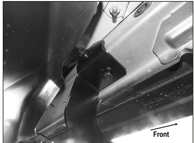
(Fig 3) Driver Front Mounting Bracket Installed
