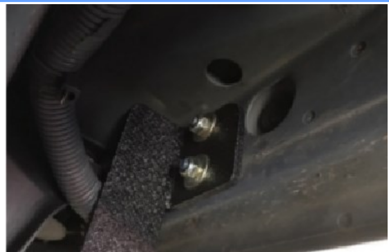
(Fig 3) Driver Side Front Mounting Bracket Installed
