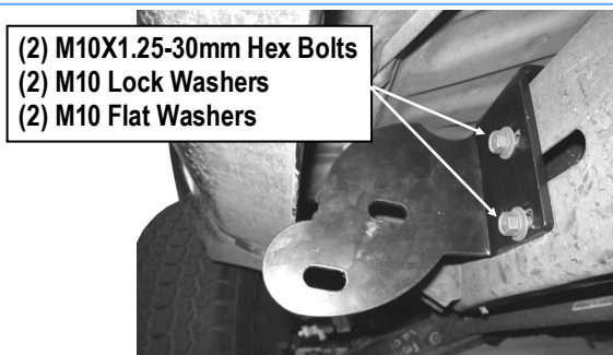
(Fig 2) Driver Front Mounting Bracket (DFM) Installed
