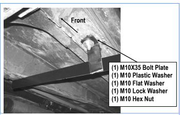
(Fig 5) Driver Side Front Support Bracket Installation (Front View Shown)
