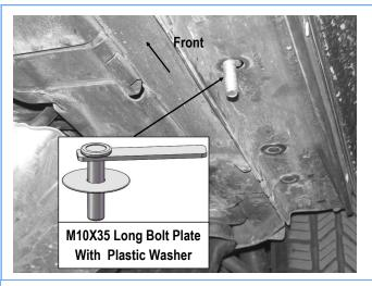
(Fig 7) Insert The M10X35 Bolt Plate
