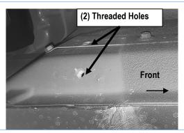
(Fig 2) 2016-On Driver Side Rear Mounting Location Pictured.
