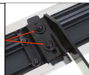
(Fig 16) Step Bar Installed on Bracket Installed (Example)
