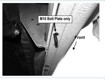
(Fig 9) Passenger Rear Mounting Bracket (PRM) Location
