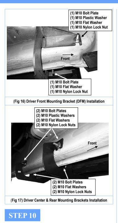
Select the Driver Side Running Board (the Short one). Repeat **Step 7** to attach Running Board to the (3) Brackets.
