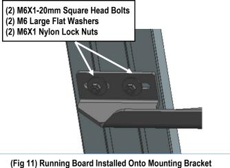
(Fig 11) Running Board Installed Onto Mounting Bracke (Example)
