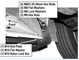
(Fig 14) Passenger Rear Mounting Bracket Complete Installation
