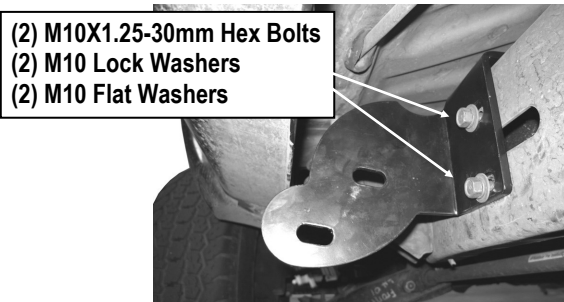
(Fig 2) Driver Front Mounting Bracket (DFM) Installed
