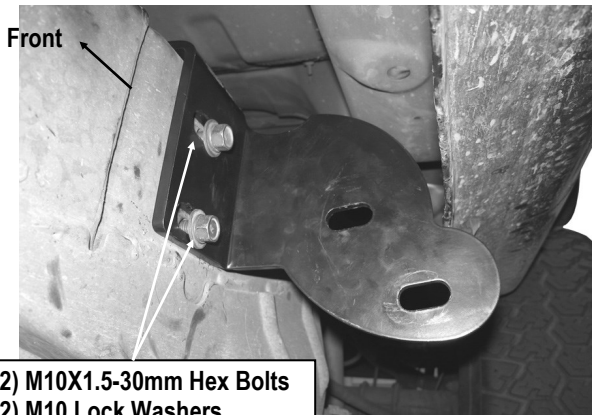
(Fig 6) Driver Rear Mounting Bracket (DRM) Installed
