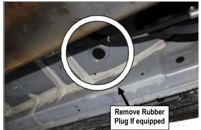
(Fig 3) Passenger Rear Mounting Bracket Installation
