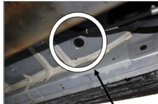
(Fig 3) Remove Rubber Plug
