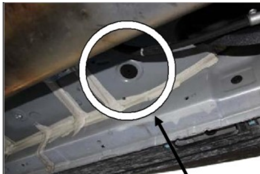
(Fig 3) Remove Rubber Plug
