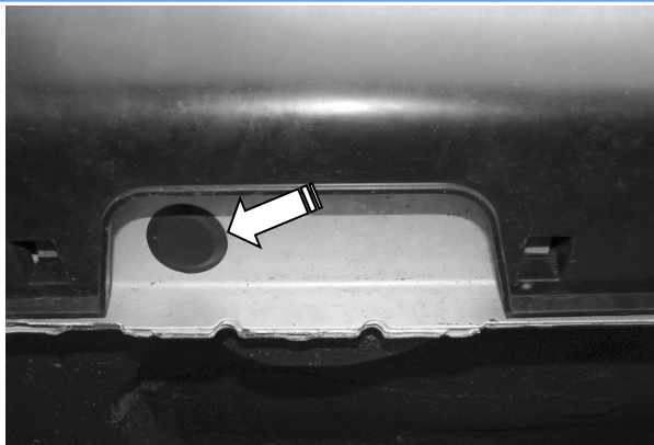
(Fig 2) Remove The Rubber Plug
