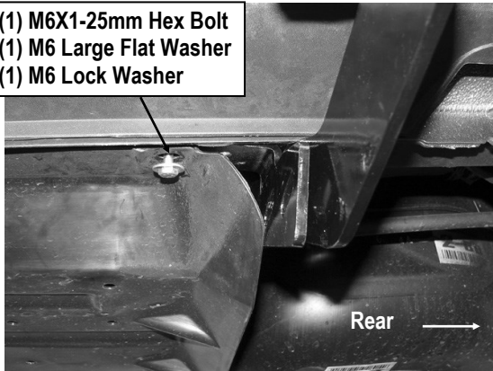
(Fig 9) Driver Rear Support Bracket Installation
