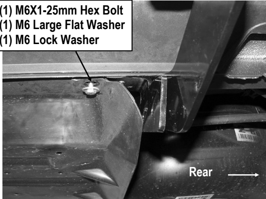
(Fig 9) Driver Rear Support Bracket Installation
