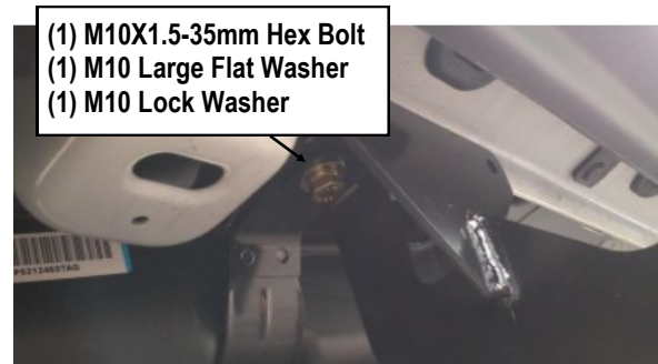
(Fig 8) Driver Rear Mounting Bracket Installed
