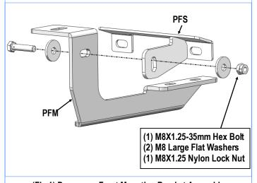
(Fig 1) Passenger Front Mounting Bracket Assembly
