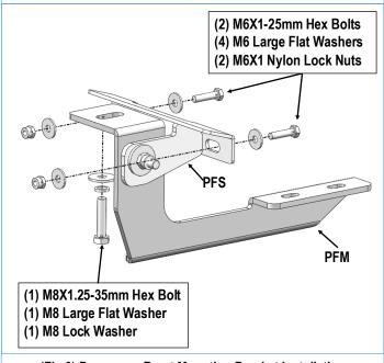
(Fig 3) Passenger Front Mounting Bracket Installation
