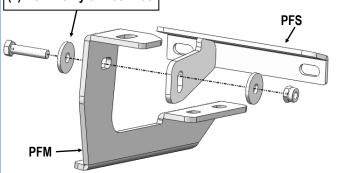
(Fig 5) Passenger Rear Mounting Brackets Assembly
