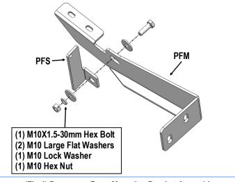
(Fig 4) Passenger Front Mounting Bracket Assembly
