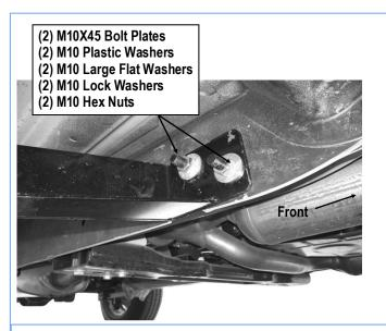
(Fig 3) Passenger Front Mounting Bracket Installation
