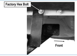
(Fig 5) Passenger Front Support Bracket Installation
