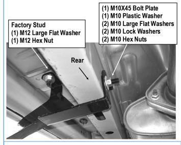
(Fig 6) Passenger Rear Mounting Bracket Installation
