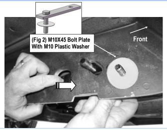
(Fig 1) Passenger Side Front Mounting Location
