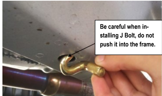
(Fig 4) Install M10 J-Bolt (On Driver Side Front Mounting Location)
